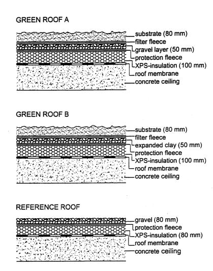
Fig. 2 Composition of the inverted roofs with greenery which have a drainage layer of gravel (A) or expanded clay (B) above the insulation and composition of the reference roof.
