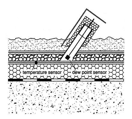
Fig. 3 Schematic picture of the installation of the sensors in the green roof.
